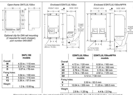
Dimensions for reference only. Use actual product for mounting template. For safe heat dissipation, mount product in orientation shown, with minimum air-gap clearance of 40mm / 1.5 in. above/below and 25mm / 1.0 in. at each side.
